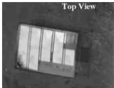
Figure 3. Membrane-supported coplanar waveguides of different lengths (line width = 50 \mu\text{m} , gap = 40 \mu\text{m} , membrane thickness < 5 \mu\text{m} , membrane distance away from ground = 110 \mu\text{m} );
