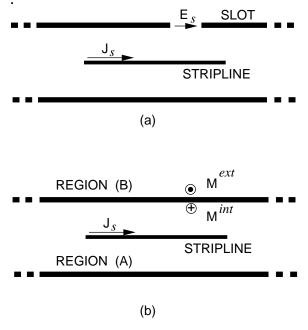
Fig. 9. Single slot-stripline-slot cell: (a) original structure; and (b) the structure after application of the equivalence principle.
