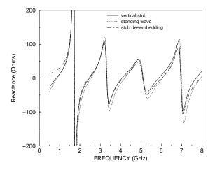
Fig. 13. Reactance of single slot circuit.
