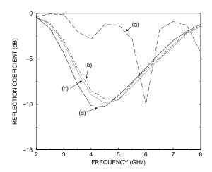
Fig. 11. Return loss of a single slot antenna using: (a) $Z_{DIFF}$ ; (b) $Z_{PORT}$  extracted using stub de-embedding; and (c)  $Z_{PORT}$  after [23]. Referring to 6  $l_L = 50mm$ ,  $W_L = 2.5mm$ ,  $l_S = 30mm$ ,  $W_S = 2mm$ ,  $l_{OFF} = 10mm$ , h = 1.57mm, and  $\epsilon_r = 2.2$ .
