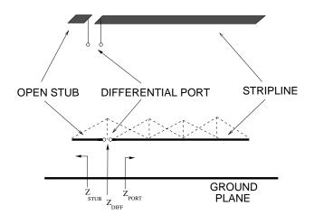
Fig. 7. Port definition for differential port and the differential bases cells.
