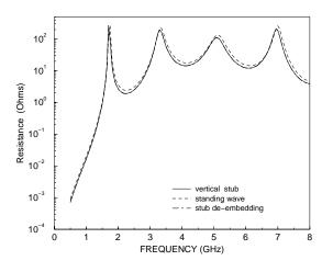
Fig. 12. Resistance of single slot circuit.
