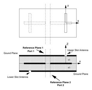
Fig. 4. Slot-stripline-slot (SSS) unit cell.
