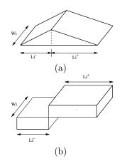
Fig. 10. Basis function: (a) rooftop and (b) pulse doublet.
