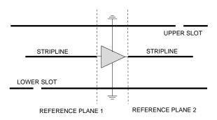
Fig. 2. Slot-stripline-slot (SSS) amplifier unit cell.
