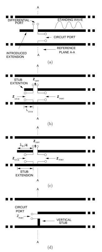
Fig. 5. Four techniques for establishing a circuit ports in MoM analysis: (a) standing wave characterization; (b) stub-de-embedding;(c) quarter wavelength stub; and (d) Vertical stub.
