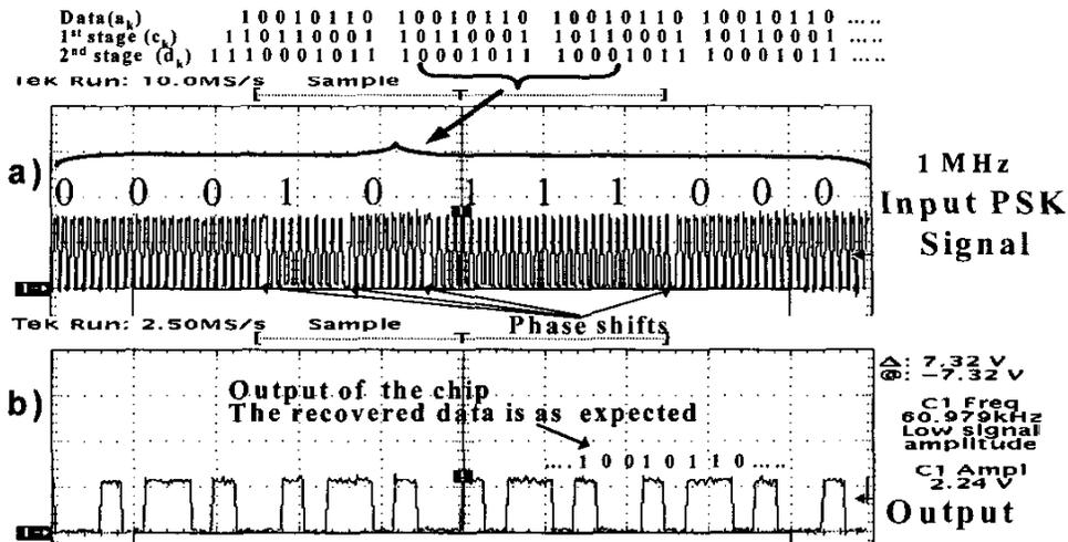
Fig. 9. The measured baseband output a) the input PSK signal-after two stage differential encoder b) the recovered data ( $= a_k$ )
