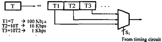
Fig. 4. Delay units in digital DDPSK for different bit rates
