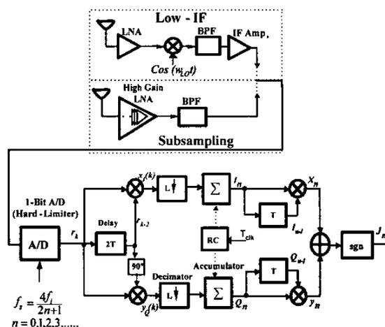
Fig. 1. Digital double DPSK receiver with the two front-ends
