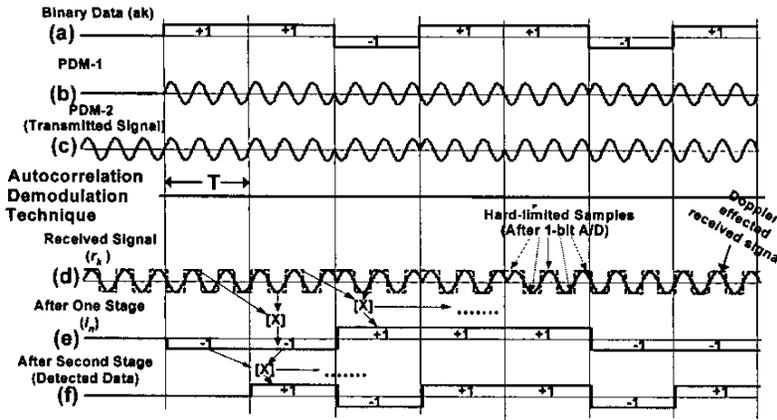
Fig.5 Timing diagram of autocorrelation techniques for digital DDPSK receiver
