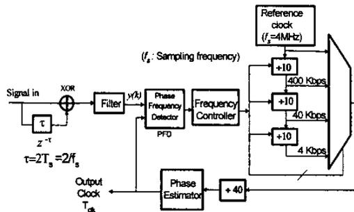
Fig. 6. Timing circuit for multiple bit rates
