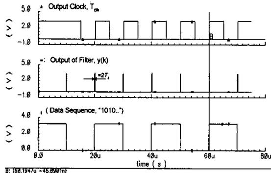
Fig. 7. Recovered timing clock for a data sequence of 100 Kbps.
