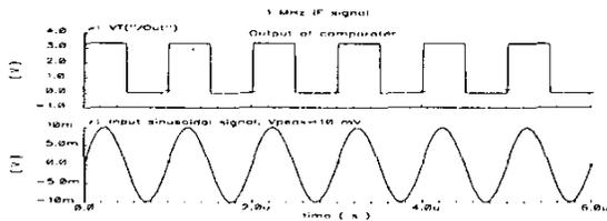
Fig. 3. 1 MHz IF signal converted to digital waveform by A/D
