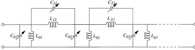
Fig. 6.  $n$ th-order filter prototype realizing arbitrarily located transmission zeros with one zero at dc, one zero at infinity, and  $(n - 1)$  zeros at finite frequencies.
