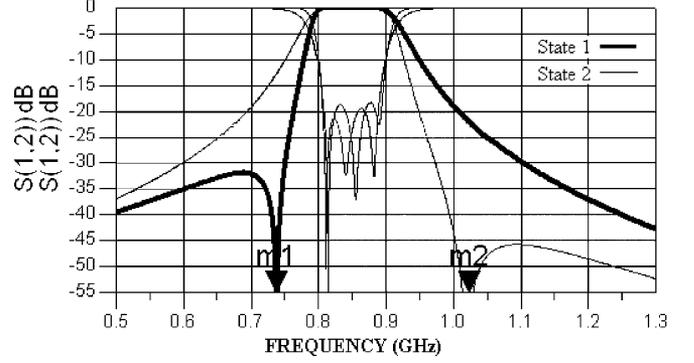
Fig. 8. Simulated lossless responses of the prototype of Fig. 7(b) in two states for the same inter-resonator couplings and RL level. (m1: 735.6 MHz; m2: 1016.25 MHz).
