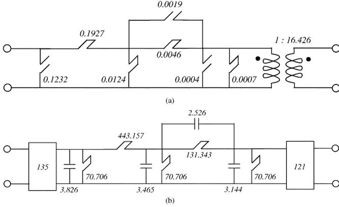
Fig. 7. Distributed bandpass filter prototype with one zero at dc, three zeros at infinity, and one zero at 735.6 MHz. (a) After direct synthesis in a 1- $\Omega$  system. (b) After application of suitable circuit transformations and scaling in a 50- $\Omega$  system. (All capacitor values are in picofarads.)
