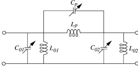
Fig. 5. Pair of bandpass resonators of Fig. 3 with mixed-type coupling.
