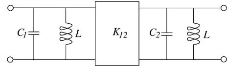
Fig. 3. Pair of bandpass resonators coupled by an impedance inverter.
