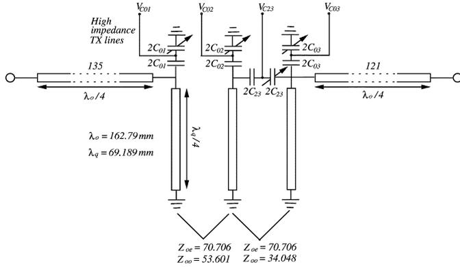
Fig. 9. Layout of combline filter based on the prototype of Fig. 7(b) with bias arrangement. (Half of the capacitors are tunable.)
