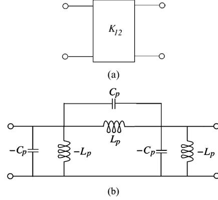
Fig. 4. Equivalence between: (a) an ideal impedance inverter and (b) its approximate model with an attenuation pole at a finite frequency.
