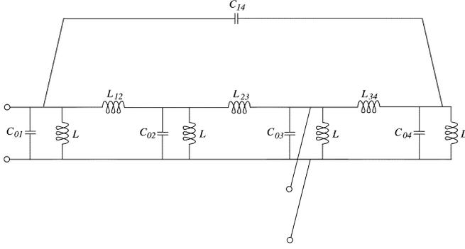
Fig. 2. Bandpass fourth-order network section realizing a single transmission zero either in the lower or upper stopband with inductive inter-resonator coupling and capacitive crosscoupling.
