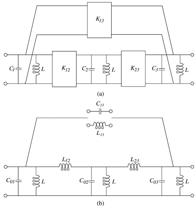
Fig. 1. Bandpass CT realizing a single transmission zero either in the lower or upper stopband: (a) with inter-resonator inverter couplings and (b) with inductive inter-resonator coupling and either inductive or capacitive cross-coupling.
