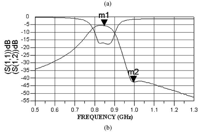
Fig. 10. Measured scattering parameters of reconfigurable filter with a finite transmission zero: (a) in the lower stopband (m1: 850 MHz,  $-5.253$  dB; m2: 732 MHz,  $-33.027$  dB) and (b) in the upper stopband (m1: 850 MHz,  $-5.753$  dB; m2: 996 MHz,  $-42.785$  dB).
