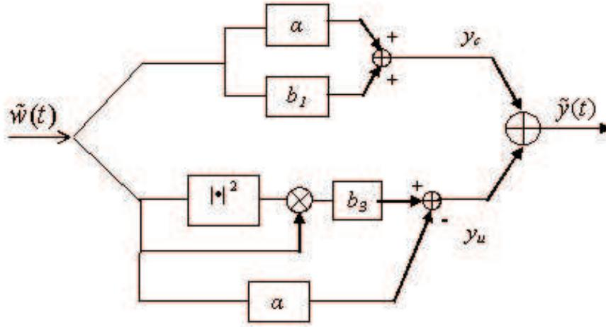
Fig. 3. Envelop nonlinear model with uncorrelated outputs.
