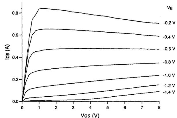
Fig. 4. Electro-thermally simulated I-V characteristics of the 10-finger Filtronic power HEMT with 6  $\mu\text{m}$  surface metallisation and adiabatic surface boundary conditions. Finger width 400  $\mu\text{m}$ ; substrate thickness 75  $\mu\text{m}$ ; heatsink temperature 300 K.
