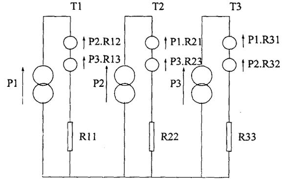
Fig. 3. Thermal circuit corresponding to resistance matrix  $R_{ij}$ .
