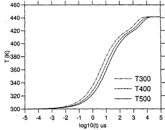
Fig. 1. Temperature rise with time at turn-on, in the immediate vicinity of the device active region in a central square,  $0.1L \times 0.1L$ , on the surface of cubic die, side  $L = 300, 400, 500 \mu\text{m}$ , dissipating 0.3, 0.4, 0.5 W.
