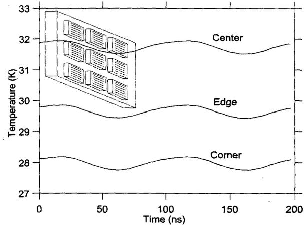
Fig. 6. Single-tone harmonic balance simulation of a power FET array (inset) representative of one kind of spatial power combining architecture. The global simulation is electro-thermally self-consistent. Heat loss is entirely by linearised radiation and convection into free space, with no heatsink mounting.
