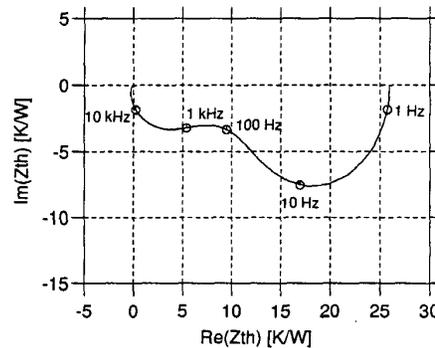
Fig. 2. Complex locus of the thermal transfer impedance, calculated using an analytical series expression, for a 4-layer, heatsink mounted structure examined by Szekely *et al.*
