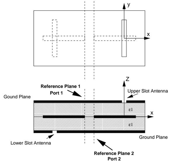
Fig. 4. Slot-stripline-slot (SSS) unit cell.
