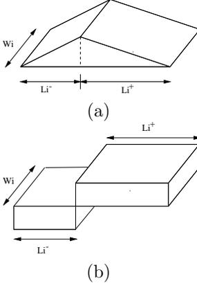
Fig. 10. Basis function: (a) rooftop and (b) pulse doublet.
