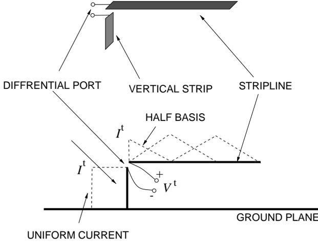
Fig. 8. Port definition for a unit cell using vertical current cell and half cell.
