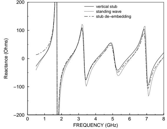
Fig. 13. Reactance of single slot circuit.
