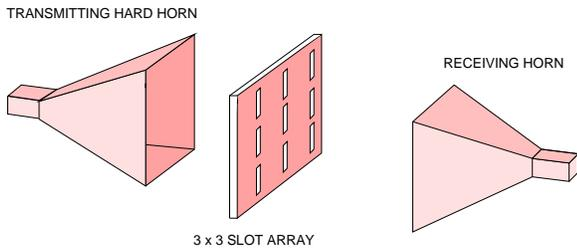
Fig. 1. A slot-stripline-slot spatial power combining system, showing a simplified  $3 \times 3$  array.
