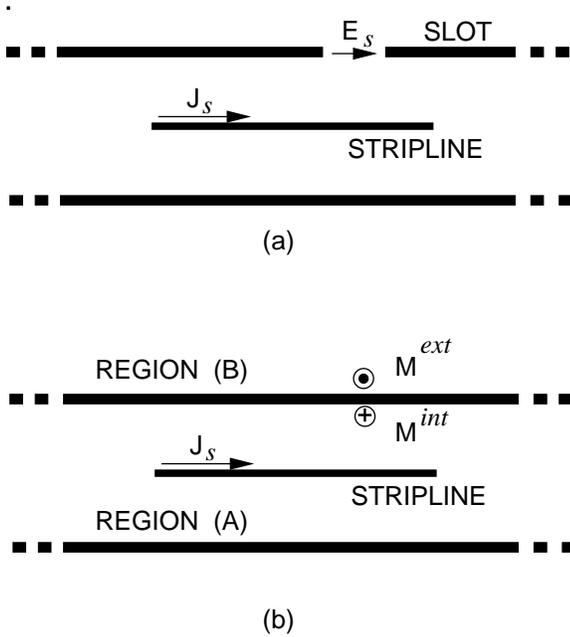
Fig. 9. Single slot-stripline-slot cell: (a) original structure; and (b) the structure after application of the equivalence principle.
