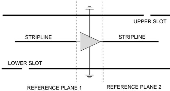
Fig. 2. Slot-stripline-slot (SSS) amplifier unit cell.
