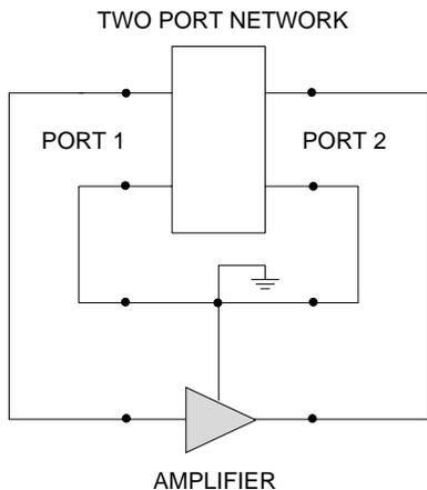
Fig. 3. Slot-stripline-slot (SSS) unit cell equivalent network.
