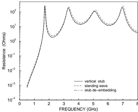
Fig. 12. Resistance of single slot circuit.
