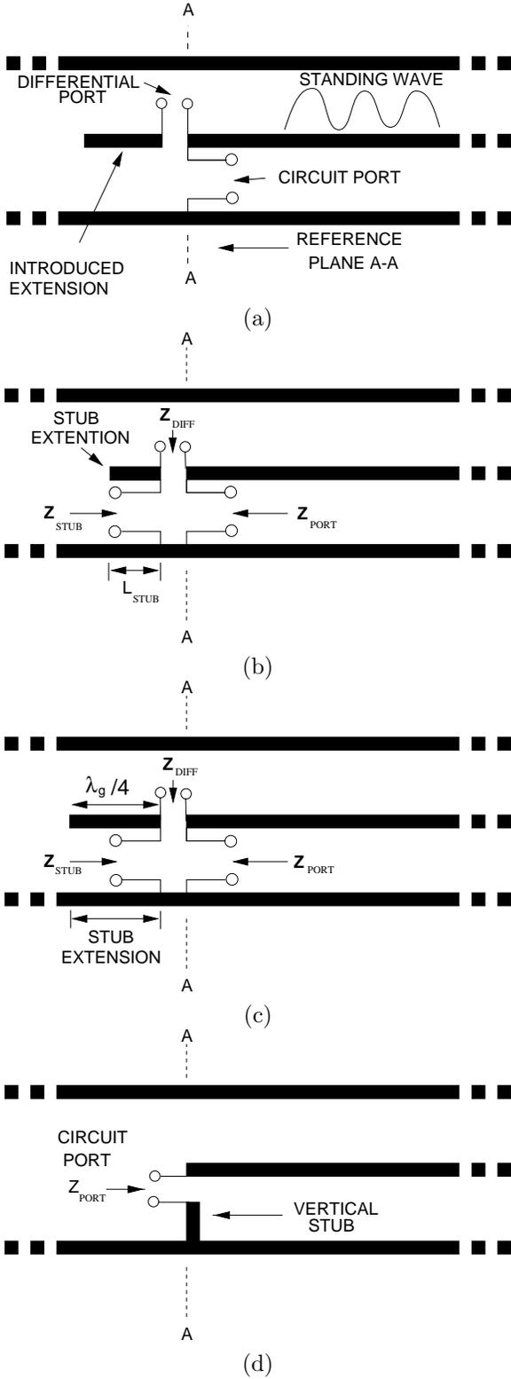
Fig. 5. Four techniques for establishing a circuit ports in MoM analysis: (a) standing wave characterization; (b) stub-de-embedding; (c) quarter wavelength stub; and (d) Vertical stub.
