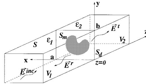
Fig. 1. Geometry of a planar arbitrarily shaped metallization in a shielded layered guided-wave structure.
