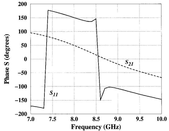
Fig. 8. Phase of  $S_{11}$  and  $S_{21}$  for the patch array embedded in a rectangular waveguide.
