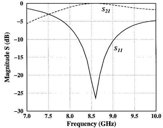
Fig. 7. Magnitude of  $S_{11}$  and  $S_{21}$  for the patch array embedded in a rectangular waveguide.
