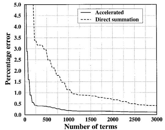
Fig. 4. Percentage error in the convergence of  $Z_{xx}$  matrix elements for the accelerated and direct double series summation.
