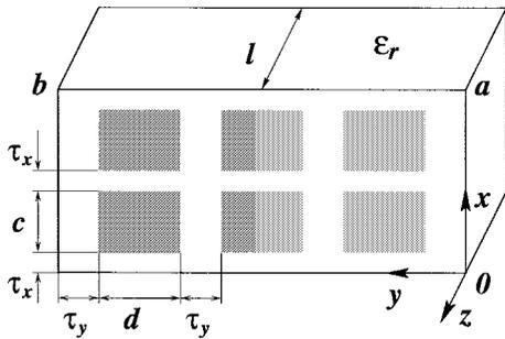
Fig. 6. Geometry of patch array supported by dielectric slab in a rectangular waveguide:  $a = 1.0287$  cm,  $b = 2.286$  cm,  $l = 2.5$  cm,  $\epsilon_r = 2.33$ ,  $d = 0.4572$  cm,  $c = 0.3429$  cm,  $\tau_x = 0.1143$  cm,  $\tau_y = 0.2286$  cm.
