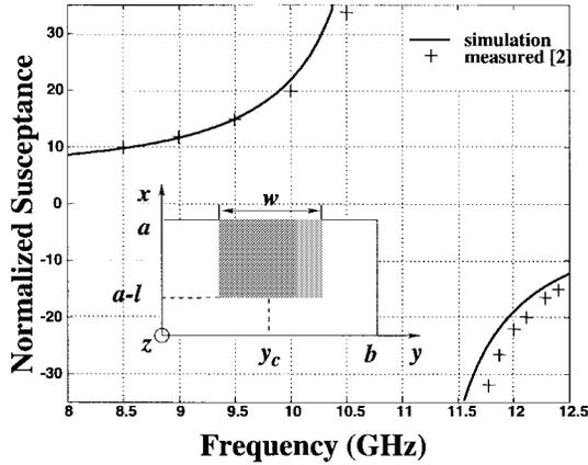
Fig. 5. Normalized susceptance of a wide resonant strip in waveguide:  $a = 0.4$  in,  $b = 0.9$  in,  $w = 0.280$  in,  $l = 0.365$  in,  $y_c = b/2$ .
