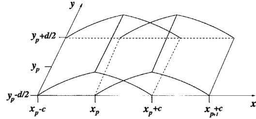
Fig. 2. Rectangular cells with the  $x$ -directed overlapping piecewise sinusoidal basis functions.
