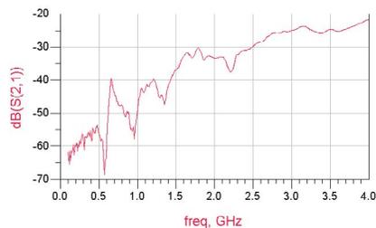
Figure 17: Crosstalk between two 3mm outer diameter inductors spaced 0.65mm apart
