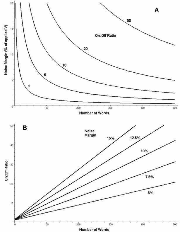
Figure 3: (a) Achievable noise margin vs. memory size for various on:off ratios (b) Required on:off ratio vs. memory size for various noise margins
