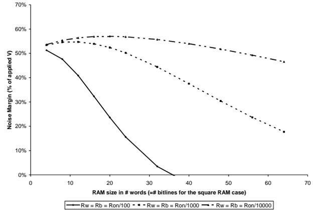
Figure 4: Scalability of fully molecular RAM for different system parameters
