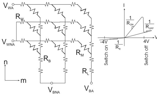
Figure 1: Molecular Random Access Memory and molecular current-voltage characteristic
