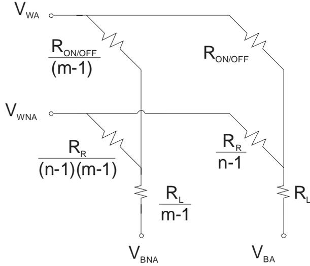
Figure 2: Circuit Template parameterized by RAM size
