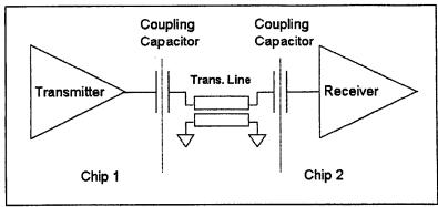
Figure 2: Schematic view of capacitively-coupled AC interconnection
