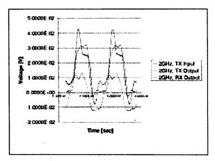
Figure 4: Measured 2GHz waveform (4Gbps NRZ) of capacitively coupled system
