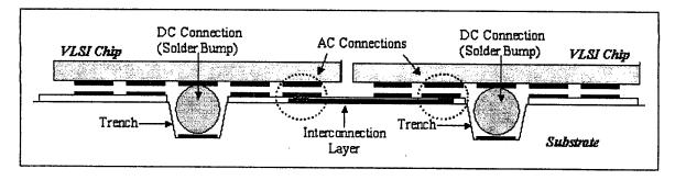
Figure 1: Cross-section of physical technology for AC Coupled Interconnection
