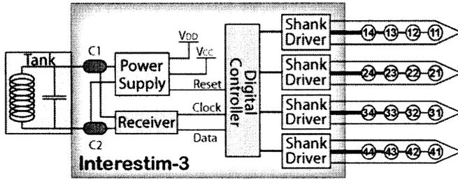
Fig. 2. Modular architecture of the Interestim-3 wireless microstimulating probe with only two interconnects (C1, C2) per probe [1].
