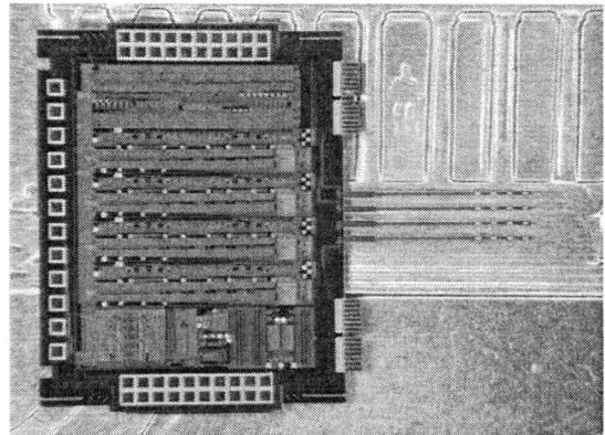
Fig. 1. Interestim-3, a 16-site micromachined planar active wireless microstimulating probe with a modular architecture [1].
